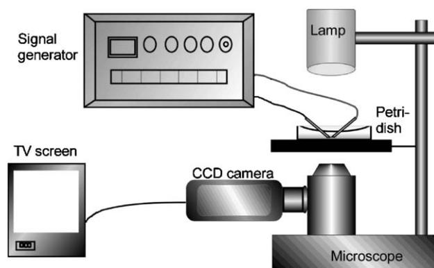
Fig. 1. A schematic representation of the experimental setup used for DEP measurements. A signal generator was used to supply an AC voltage to the electrodes. Observations were made using a video camera connected to a television and video recorder for data collection and analysis.
