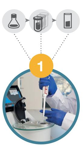
Pipette sample directly onto the pedestal
