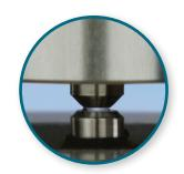
The pedestal then moves to automatically adjust for an optimal path length (0.03 – 1 mm).
