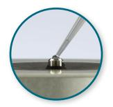
With the arm open, a sample is pipetted directly onto the pedestal.
