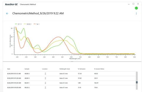
NanoDrop QC Software chemometric spectra analysis of dye samples Red – Tartrazine Green – Sunset Yellow
