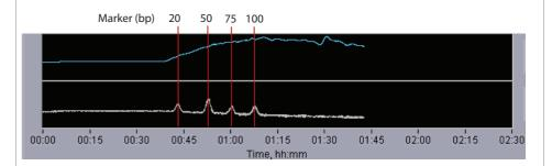
The following bioanalyzer results indicate typical results from QC testing.
