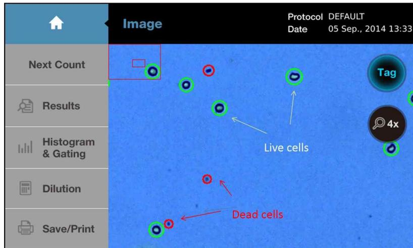
**Note:** This “Tag” function is one of the distinct tools of the LUNA-II™ Automated Cell Counter. This function allows the user to review the data immediately to determine the accuracy of the counting without additional manipulation or devices.
