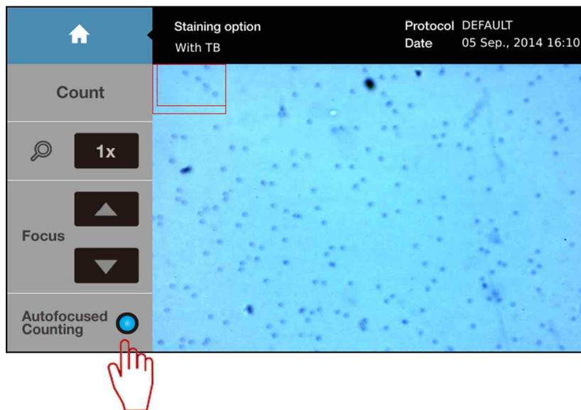
As shown above, the Luna™ Standard Beads are out-of-focus. However, users can count the beads without tedious focusing.
