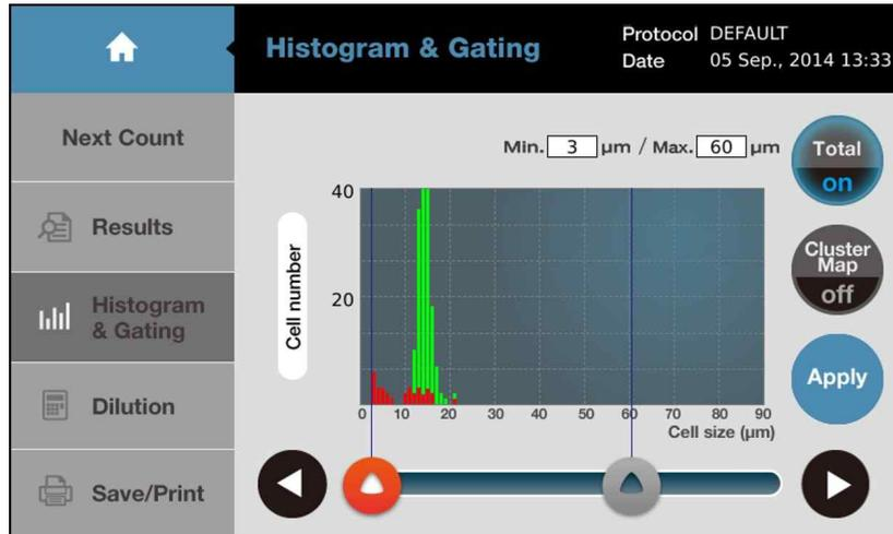
On this screen, users can review the distribution of cells according to their sizes. Green bars represent the live cells and red bars represent dead cells.
