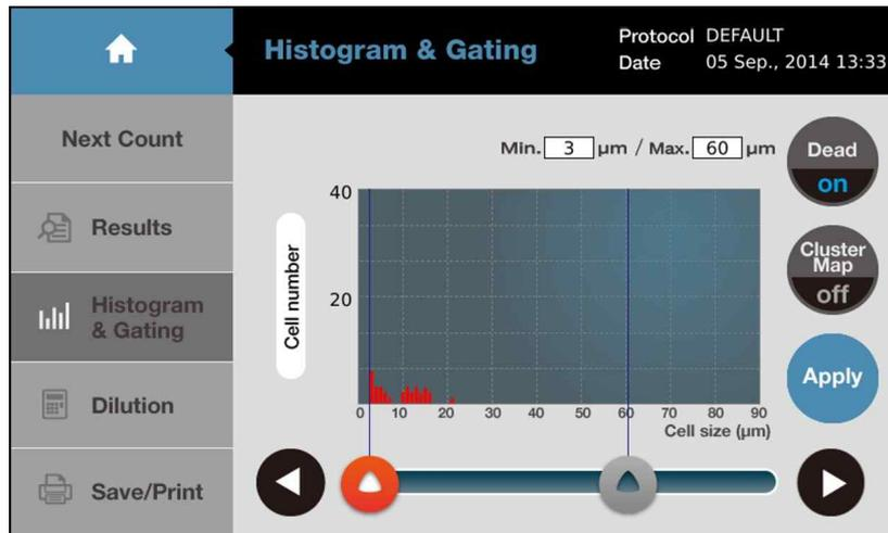
In addition, when pressing [Cell number] on the left side of histogram, the LUNA-II™ Automated Cell Counter also display the cell concentration.
