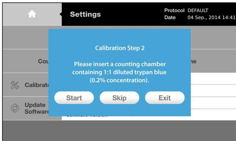
Now, place the cell counting slide containing diluted trypan blue solution into the counting slide port. Be sure the chamber containing the trypan blue solution to be placed inside the instrument. Do not turn the cell counting slide upside-down.
