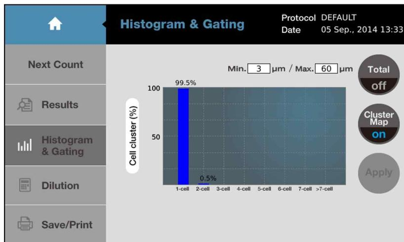
In addition, the LUNA-II™ Automated Cell Counter provides gating function. Gating function consists of four components: the lower and upper limit and two arrow head in the lower part of screen as below.
