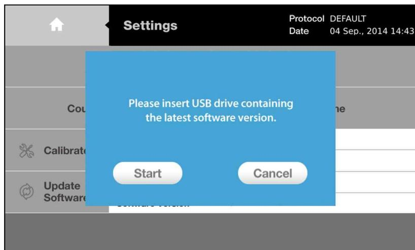
Press [Start]. Software update will be proceeded automatically. Do not turn off the instrument during update. After finishing, the current version of software and the date of last update will be changed automatically.
