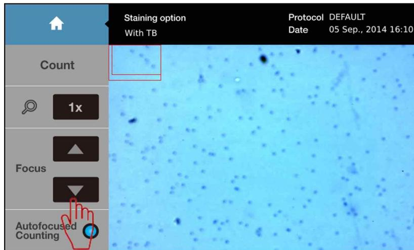
**Note:** If needed, users can count the cells with deactivating autofocus function after manual focusing.
