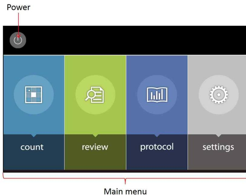
The Power icon in the Start-Up screen can be used to turn off the instrument. See Section 7.1. for further information to turn on/off the instrument.
