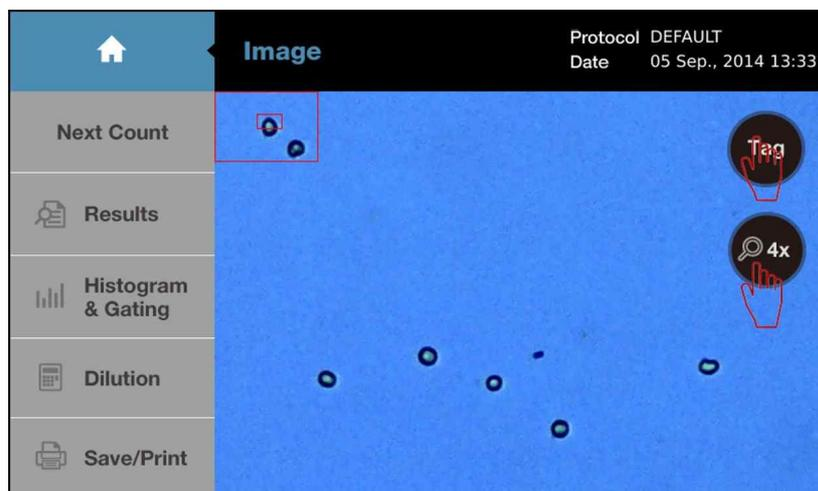
Similar to the Count screen, the magnification of the captured image can be changed by pressing the magnifier button on the right of the image. The LUNA-II™ Automated Cell Counter provides 1X, 2X, and 4X magnification of the image.
