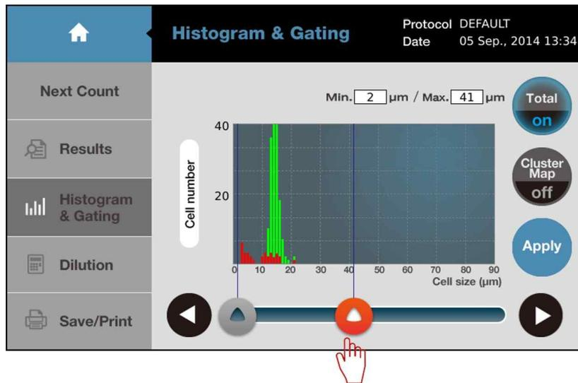
The lower and upper limit can be activated by pressing as above and adjusted by pressing the icons with arrow head.
