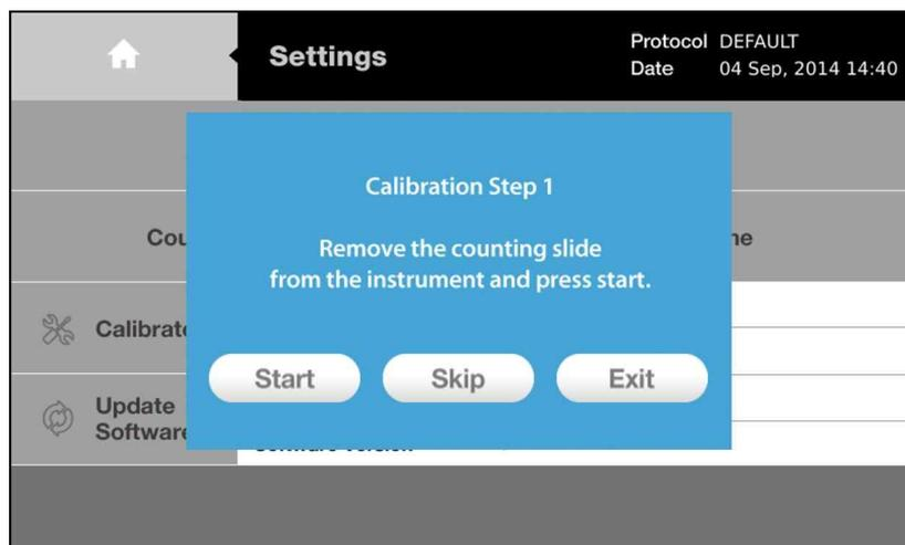
For the Calibration Step 1, the counting slide port should be emptied. As directed on the screen, remove the counting slide from the counting slide port of the instrument. Press [Start].
