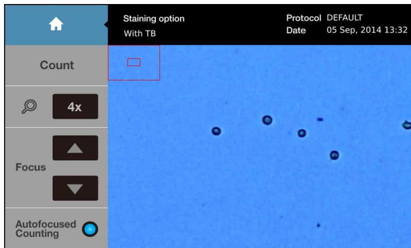
The field of cell image can be navigated by pressing the screen and moving the finger or stylus pen on the image. Two small red boxes in the upper left corner of cell image represent the entire field and field of view, respectively. The outer box represents the entire field of image. And the inner box represents current field of view. Upon navigating the image, the location of inner box will be changed.
