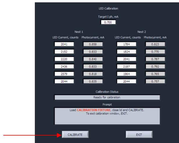
6. The LED photocurrents will automatically adjust to a factory setting, and the “Calibration Status” field will contain the message “Calibration OK”.
