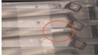
If the agarose has delaminated in the optical region, do not use that lane to run the reference marker.
