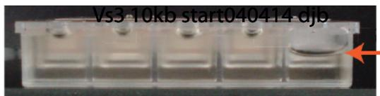
If a buffer reservoir is low, fill with spare buffer.
