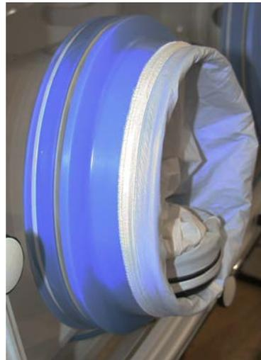
**Note:** As the O-rings are designed to fit tightly over the sleeve to create an effective seal, they can be difficult to fit. It is recommended that prior to fitting, the O-rings should be stretched several times to warm up the rubber to make it more compliant.
