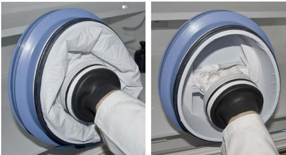
The Sleeve should pull forcefully against both the inner surface of the Glove port interior and the users arm and hand when adequate vacuum has been achieved.
