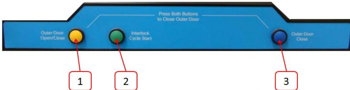
1. Outer door open / close button. Press individually to open the interlock outer door. Press the open and outer door close button (item 3) to close the interlock outer door.
