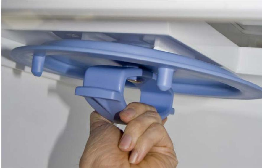
**Figure 26: Glove port cap storage location inside workstation**
