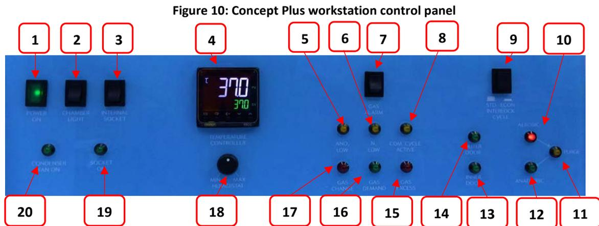
1. **Power indicator.** Illuminates to indicate the workstation is connected to the mains power supply and is switched on.
