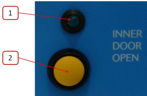
1. Inner door LED indicator. Illuminates to indicate when the interlock inner door is available.
