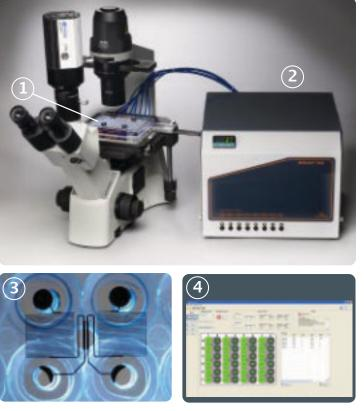
1. The Pressure Interface mounts on top of the BioFlux Plates and sits on an inverted microscope.
