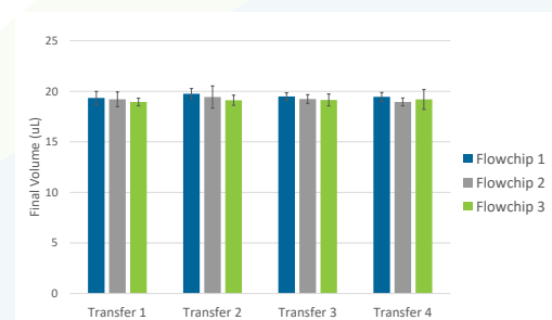
Figure 7. Fluid transfer demonstration results. Error bars represent +/- 1 SD (n=8)
