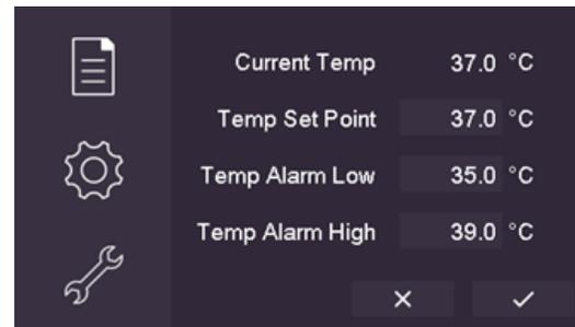
This is the Temperature setting screen, the CO<sub>2</sub> screen is similar.
