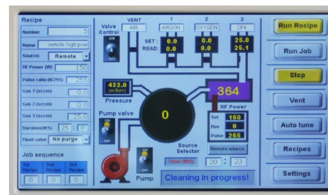
Gentle ion-free downstream mode plasma clean
