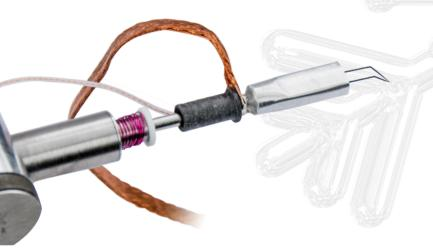
microscope 's cryo shield or cryo stage. Thus, the gripper can be cooled to LN2 temperature while the MM3A-EM remains at room temperature. This greatly reduces the thermal load for your microscope's cooling system.
