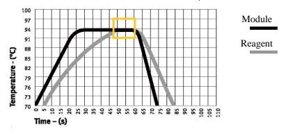
"Tube" mode considers the lagging reagent temperature ramp, and provides an overshoot process after reaching set temperature to enable reagent to reach the set temperature more quickly. If setting time equal to that of "Block" mode, the actual time for reagent reaching set temperature is obviously extended (see the figure below for the relation between module temperature and reagent temperature).
