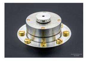
This compact device is mounted to your SEM's stage using the usual dovetail or a specialized mount, depending on the microscope in question. The only additional piece of hardware that is required is a vacuum feedthrough.
