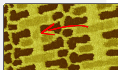
Current Imaging map on 22 nm technology The arrow indicates the location of a leaky gate...
