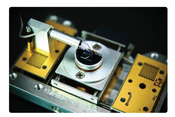
Preparation of the Lift-out Shuttle with new sample and a TEM grid is done *ex-situ*, usually with the aid of a light microscope. The entire setup is then introduce into the vacuum-ready SEM or FIB via the load-lock. The three steps described above can be repeated for multiple samples without breaking vaccum. Minimizing ven
