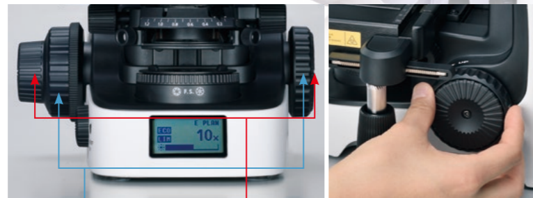
Coarse focus knob Fine focus knob Coarse/fine focus and stage movement can be operated with one hand
