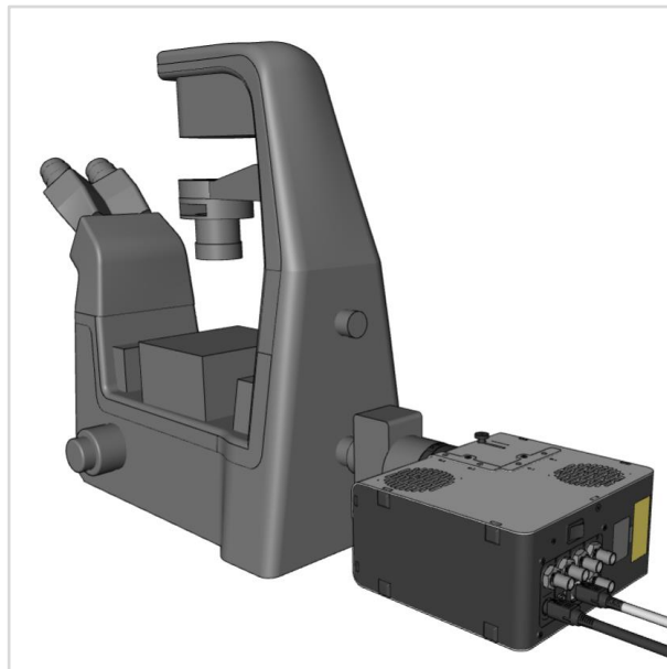
Figure 10 – A pE-400 max Light Source fitted to a microscope in a horizontal orientation.
