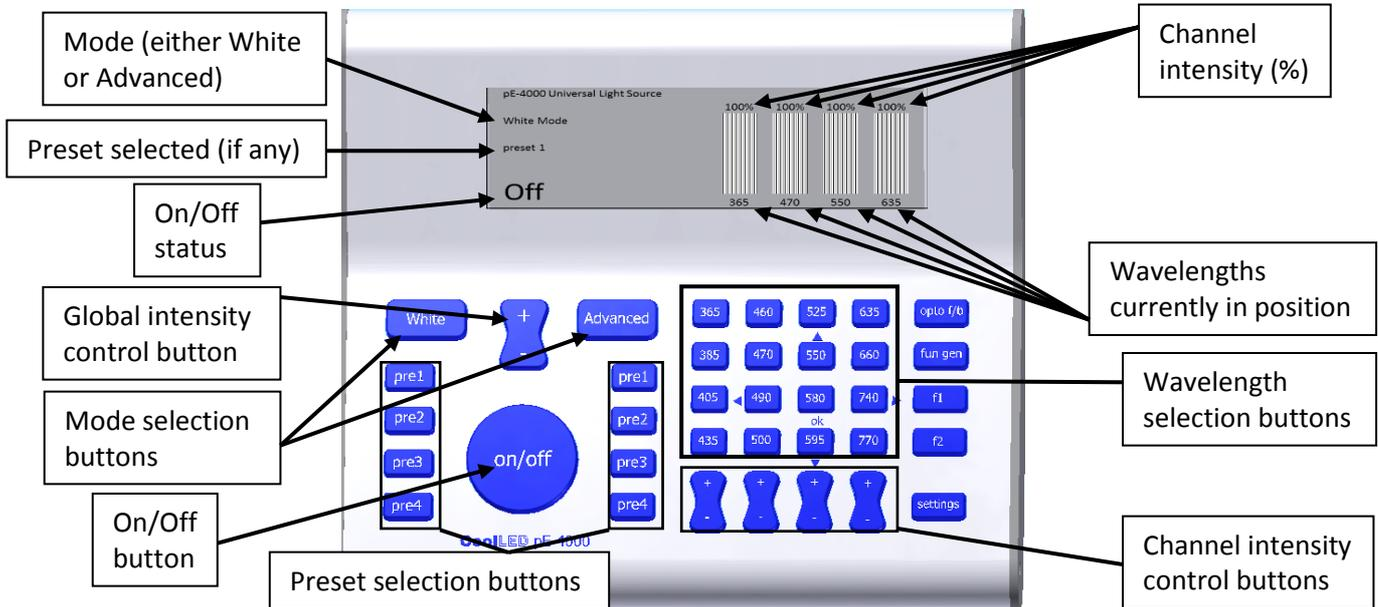
When the system is powered up the Light Source shall be in “White” mode. The only buttons that you will be able to press whilst in this mode are the On/Off button, the global intensity control button, the “White” preset buttons and the “Advanced” button.
