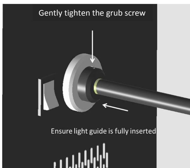
Remove the protective caps from the light guide and insert one end fully into the Light Source. Ensure that the grub screw is fully loosened to avoid any obstruction.
