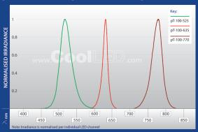
**pT-100-525** provides phosphor-free illumination centred around 525 nm, a bandwidth which is optimised for the spectral response of most scientific cameras. This allows switching between standard brightfield and fluorescence imaging without the fear of background from a phosphored LED. The pT-100-525 will allow you to achieve great contrast from both brightfield and fluorescence imaging. This variant is available with direct fit light delivery.
